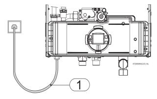
Fig. 33 Connecting power supply cord
